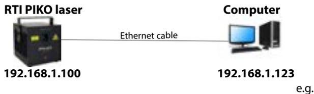
Laser device as RTI PIKO has its own default IP address 192.168.1.00. In order to establish the connection, connect the laser device through the ethernet cable directly with the laptop or PC.
