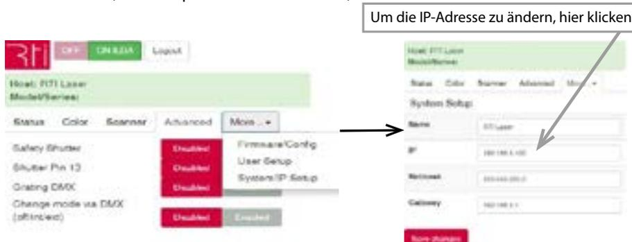
The screenshot shows the web interface of the RTI PIKO Laser. The 'More' menu is expanded, and 'System/IP-Setup' is selected. An arrow points from the 'More' button to the 'System/IP-Setup' option. Another arrow points from the 'System/IP-Setup' option to the 'IP' field in the configuration page, which is highlighted by a callout box.
